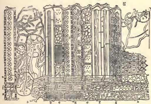
FIG. 49.—Highly magnified longitudinal radial section of a piece of oak destroyed by a timber fungus, showing the ravages of the hyphæ in the various tissues. (R. Hartig.)
